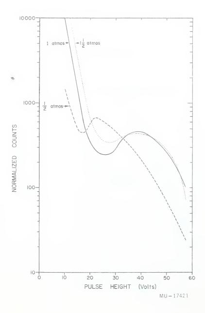
Fig. 11. Differential pulse-height spectra of the 1.05-mg/cm<sup>2</sup> chamber for gas-filling pressures of  $\frac{1}{2}$ , 1, and  $1\frac{1}{2}$  atmospheres.
